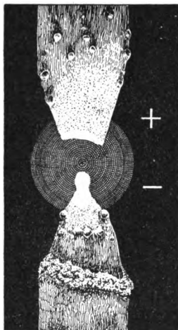
FIG. 173.— The Electric Arc.
